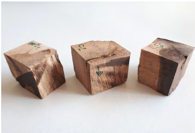
A block from a vine stock after being impregnated and densified.
