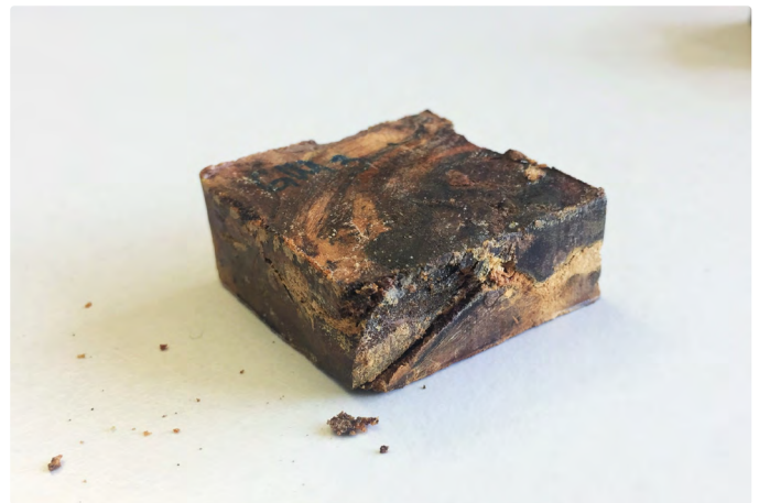
A block from a vine stock after being impregnated and densified.
